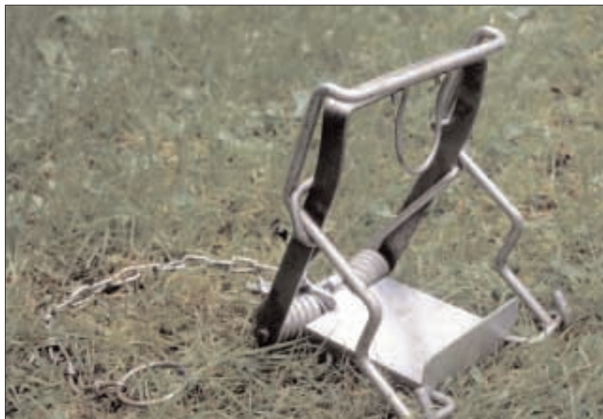
13 A Fenn Vermin Trap Mark VI – all spring traps used for rabbit control must be approved under the Pests Act 1954
