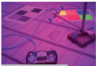
Figure 9. Measuring the wavelengths reflected by various coloured sticky traps under red and blue LEDs
