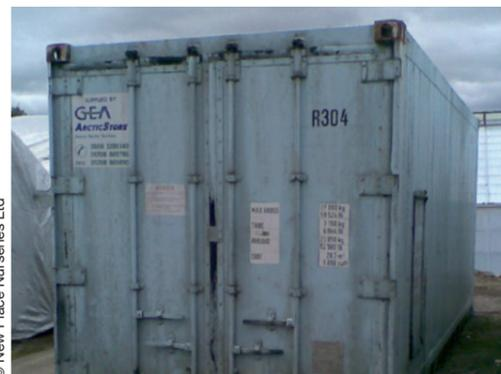
Fig 8 Refrigerated container bodies are a low cost facility which are ideal for the short-term storage of seeds and cutting material
