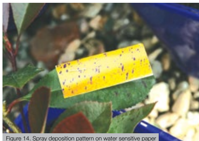
Figure 14. Spray deposition pattern on water sensitive paper
