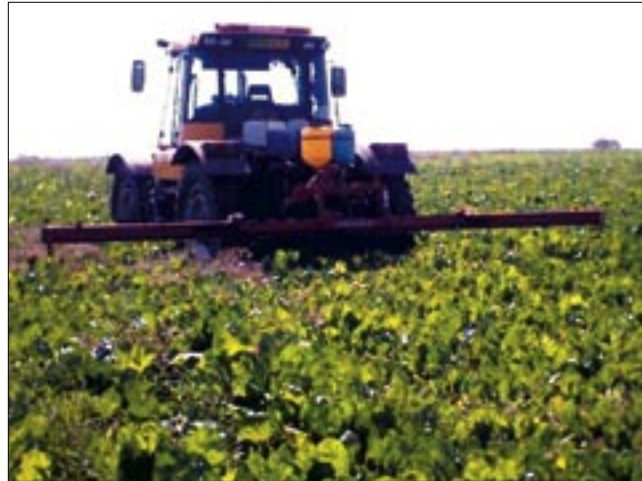
5 Weed wipers offer useful control where there is a height differential between the crop and the volunteer potatoes
