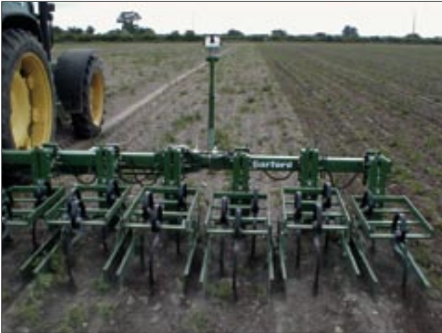
4 Precision weeding using vision-guided hoe
