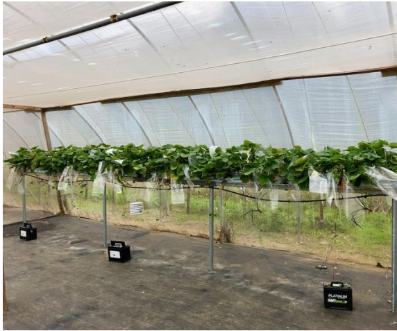
Figure 15: Trial set up showing treatment row, including insect exclusion mesh and polytunnel structure in background, batteries, data logger in a white Stevenson screen and exclusion bags on plants.
