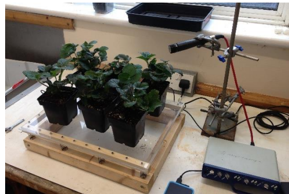
Figure 4: Laboratory set up showing vibrating platform supporting 6 potted strawberry plants (L) with microphone and audio interface (R) connected to laptop (out of shot).
