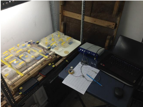
Figure 7: SWD egg laying assessment. Perspex boxes on left of image positioned on vibrating platform. Untreated control (no vibration) on white tray. Audio interface and laptop seen on table along with (disconnected) piezoelectric acoustic pick up diaphragm.
