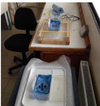
Figure 5: Apparatus testing. Treatment (top), control (bottom), each with Perspex box containing dampened blue roll and 5 blueberries in dish. SWD to be added and lids replaced.
