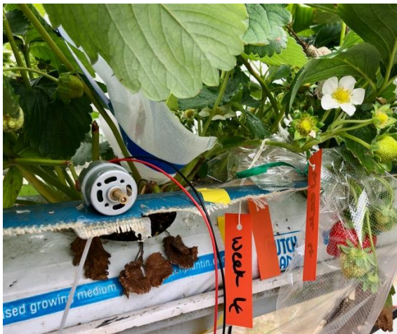
Figure 13: Adapted motor attached to treatment trellis tape using zip tie. Please note off-centre weight not visible on the axle as it is in motion. Fine mesh exclusion bag visible (above right of motor) and microperforated plastic bread bag containing ripening fruit truss to right of image. Orange labels indicate assessment number.
