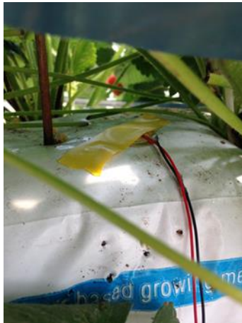
Figure 11: Piezoelectric pick up located on grow bag, between leg poles (i.e. not directly above a leg).
