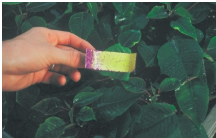
16 Water sensitive paper is an easy and simple way of quickly assessing spray coverage
