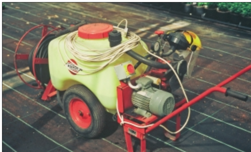
3 Small capacity HV sprayer, suitable for treating areas up to 0.5 ha
