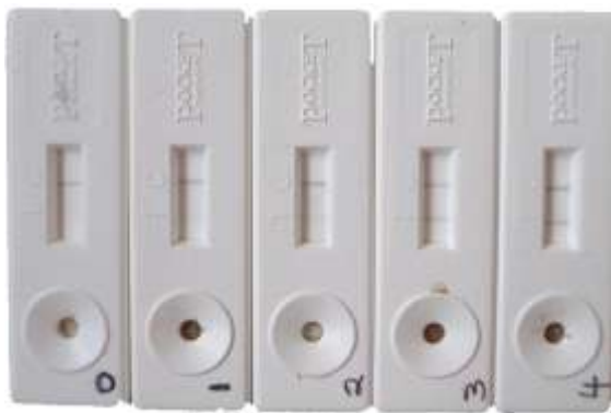
Figure GS 1: Lateral flow devices showing intensity of positive test (T) line as indexed 0 to 4 (darkest). The control (C) line indicates that the LFD is working properly.
