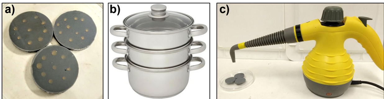
Figure 13. a) dried FOL4 chlamyospore suspension dried on polypropylene discs; b) food steamer used to treat spores, c) handheld steam cleaner used to steam treat spores.
