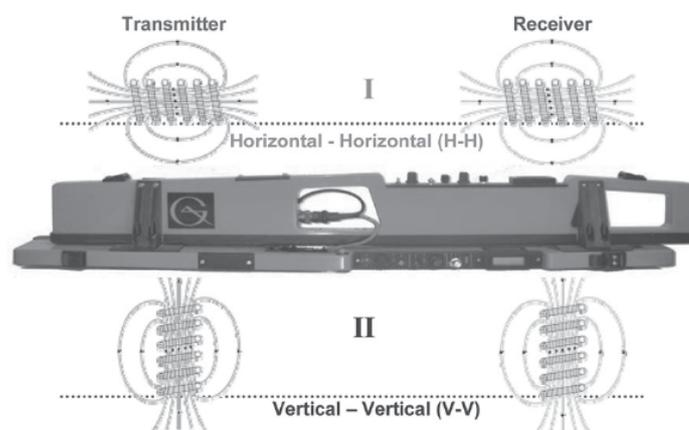
The two different transmitters and receiver coils orientations (Horizontal-Horizontal and Vertical-Vertical) allow soil scanning at different soil depths (Figure 3). The horizontal scanner has the maximum response at 0.4m depth when the instrument is carried about 50 mm above ground (James *et al.*, 2003) while the vertical scanner has a maximum response depth of approximately 1.2m. However, measurement errors caused by moving and carrying the scanner are much reduced with the deeper scan.
