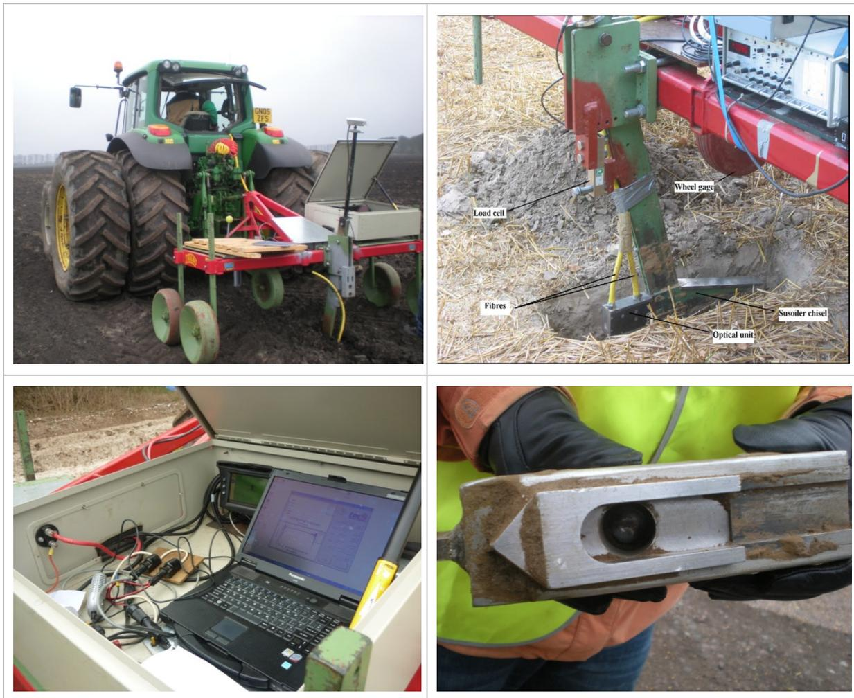
Following the on-line Vis-NIR soil scanning, 35 soil samples were randomly collected from each field in order to calibrate a Vis-NIR model for soil organic carbon and moisture content. Figure 6 provides a schematic representation of the different steps undertaken to map the different soil properties at each of the study sites.
