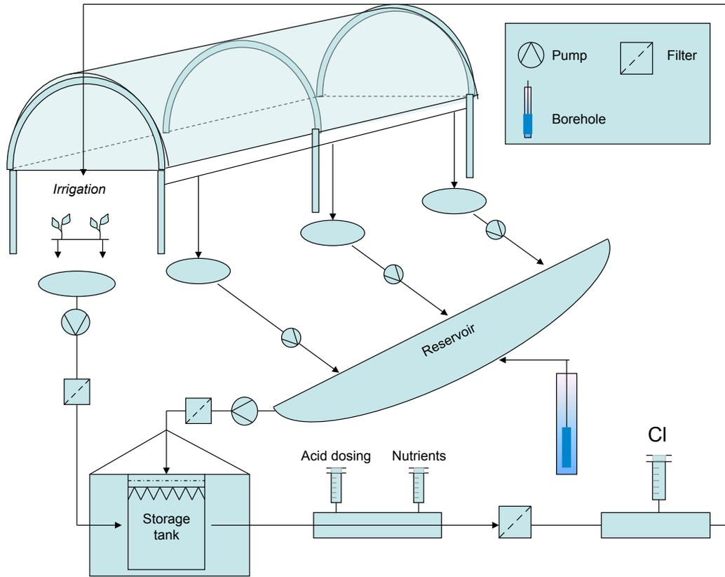
**Diagram 2. Large scale tunnel water collection and run-off collection, chlorine sterilised**
