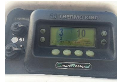
Figure 4: Controller used to set the chilled lorry temperature
