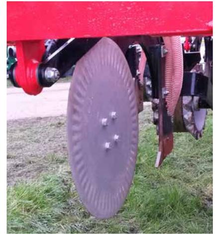
Figure 32. Examples of tine-based drills with leading discs. These enable effective operation in higher levels of residues and reduce soil disturbance
