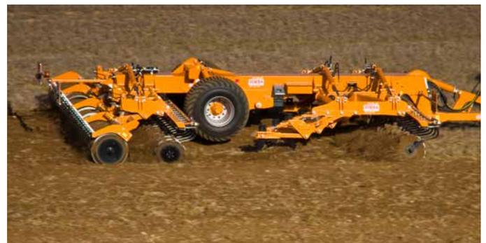
Figure 23. Typical high disturbance, deep non-inversion mixing action
