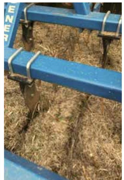
Figure 14. Geometry of loosening parts and minimal surface disturbance (left). Sufficient lift to create vertical fissures is needed at the problem depth. Low rake angles minimise surface disruption and heave, provided lift height is adequate for fissure creation. Sideways inclined legs (right) can also minimise surface disturbance, provided operational speeds are appropriate
